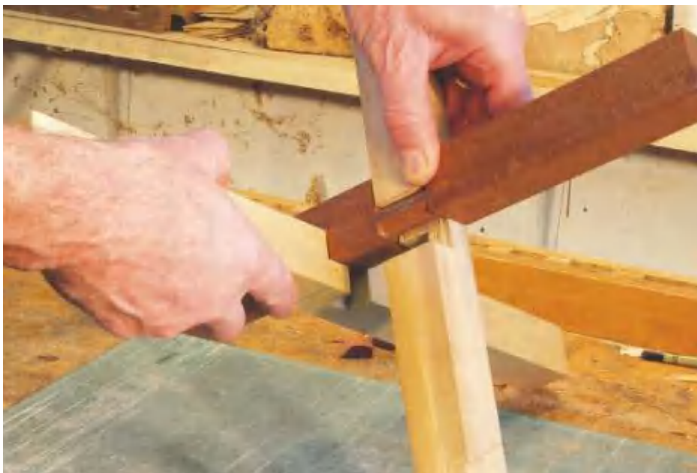
▲ Pic.15 The second piece slides along the third piece into position
